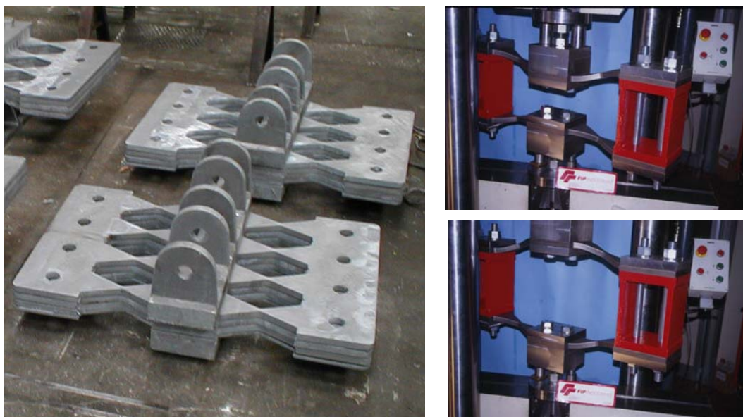
Figure 3 - X-shaped steel hysteretic dampers for a bridge in Albania undergoing assembly (left) and testing of their components (right).
